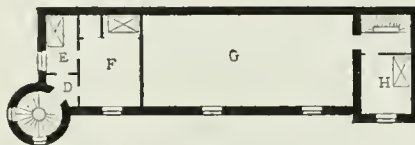
UPPER STORY: D , LANDING; E , F , H , BED ROOMS; G , FODDER LOFT.
